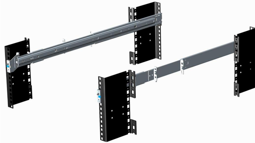
One key factor in selecting the proper rails is identifying the type of rack in which they will be installed. Both the sliding rails and the static rails support tool-less mounting in 19"-wide, EIA-310-E compliant square hole and unthreaded round-hole 4-post racks. Both also support tool-ed mounting in threaded hole 4-post racks, but only the static rails, as the more universal solution, support mounting in 2-post (Telco) racks.
