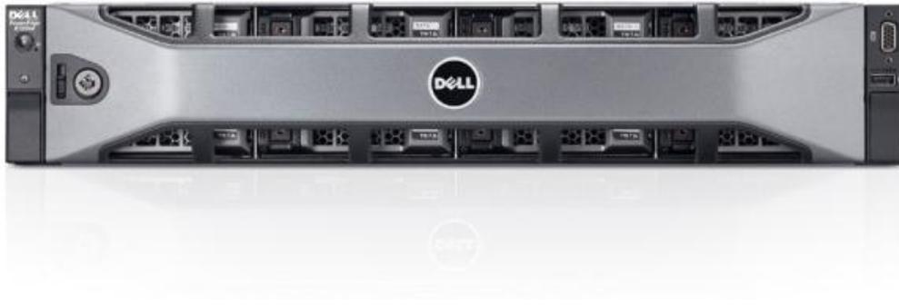
**Figure 4. R720xd front view (2.5-inch chassis without bezel)**
