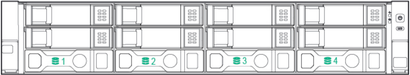
4 LFF hot-plug drive model
