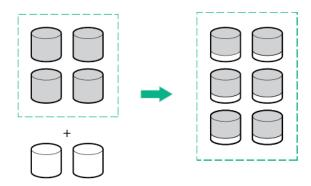
When the expansion process has finished, you can use the liberated storage capacity on the enlarged array to create new logical drives. Alternatively, you can use HPE SSA to enlarge (extend) one of the original logical drives.
