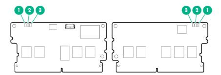
For an explanation of each of the identified components and their illumination patterns, see "FBWC LEDs illumination patterns (on page 16)."
