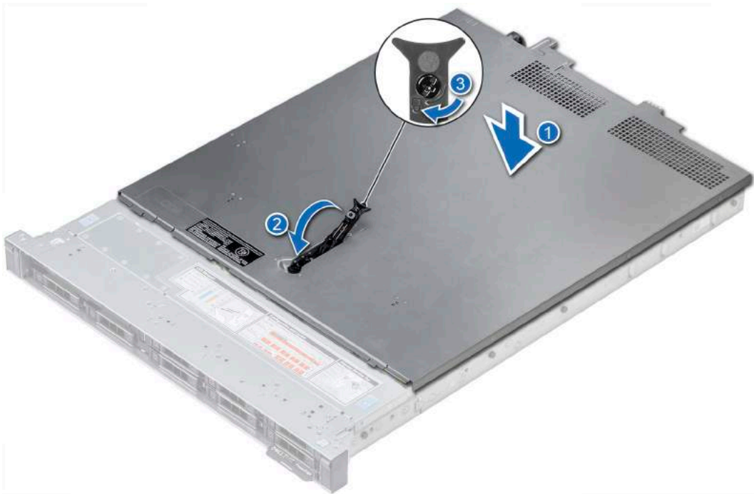
Figure 24. Installing the system cover
