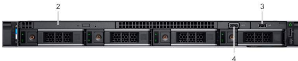
Figure 2. Front view of 4 x 3.5 inch drive system
