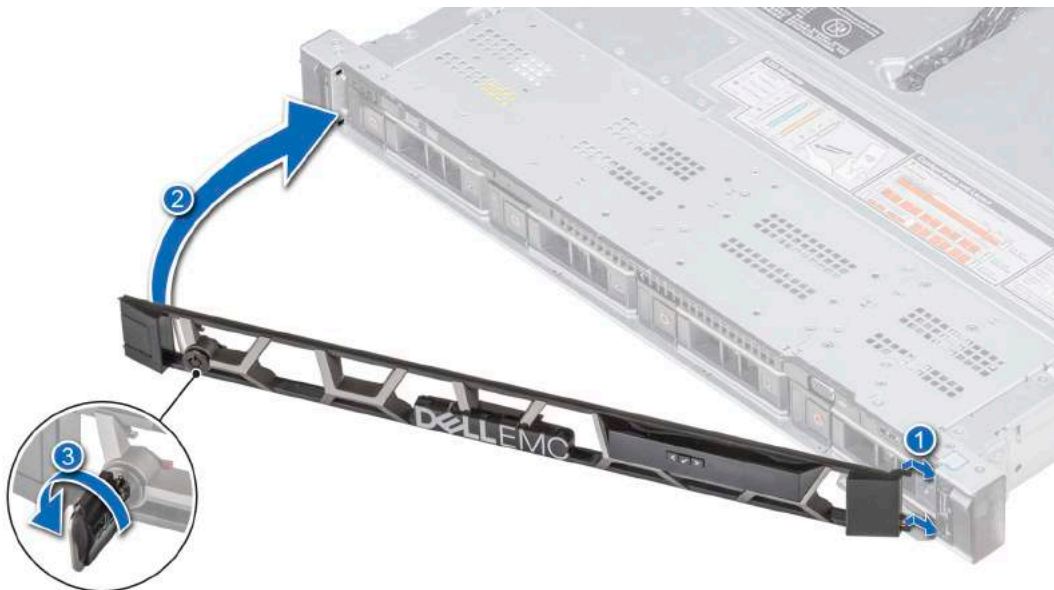
Figure 22. Installing the front bezel with the LCD panel
