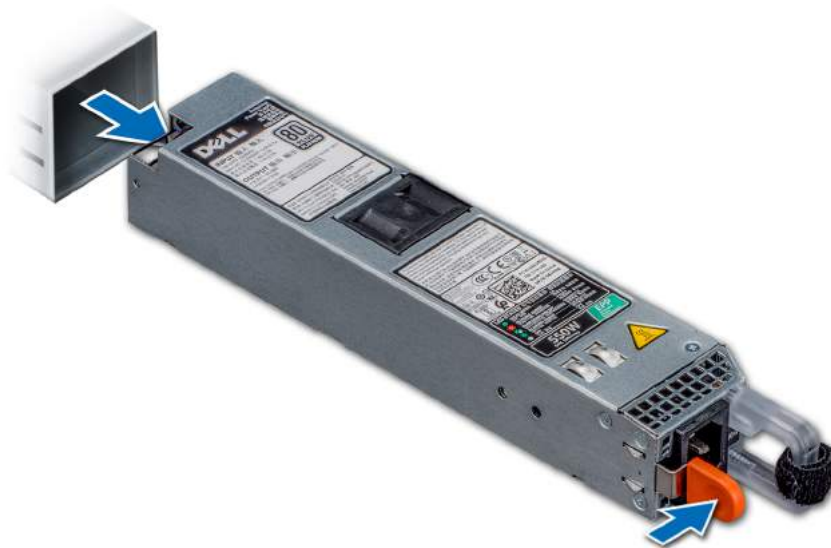
Figure 85. Removing a power supply unit
