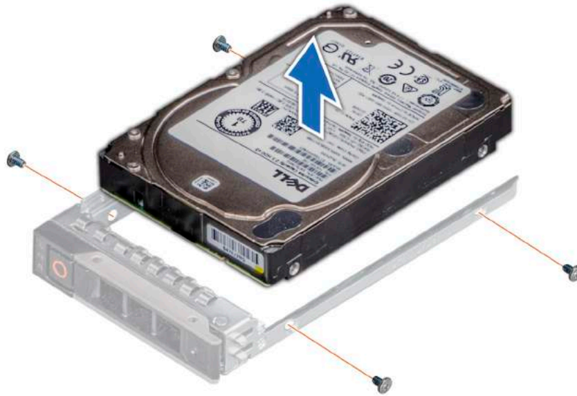
Figure 47. Removing the drive from the drive carrier
