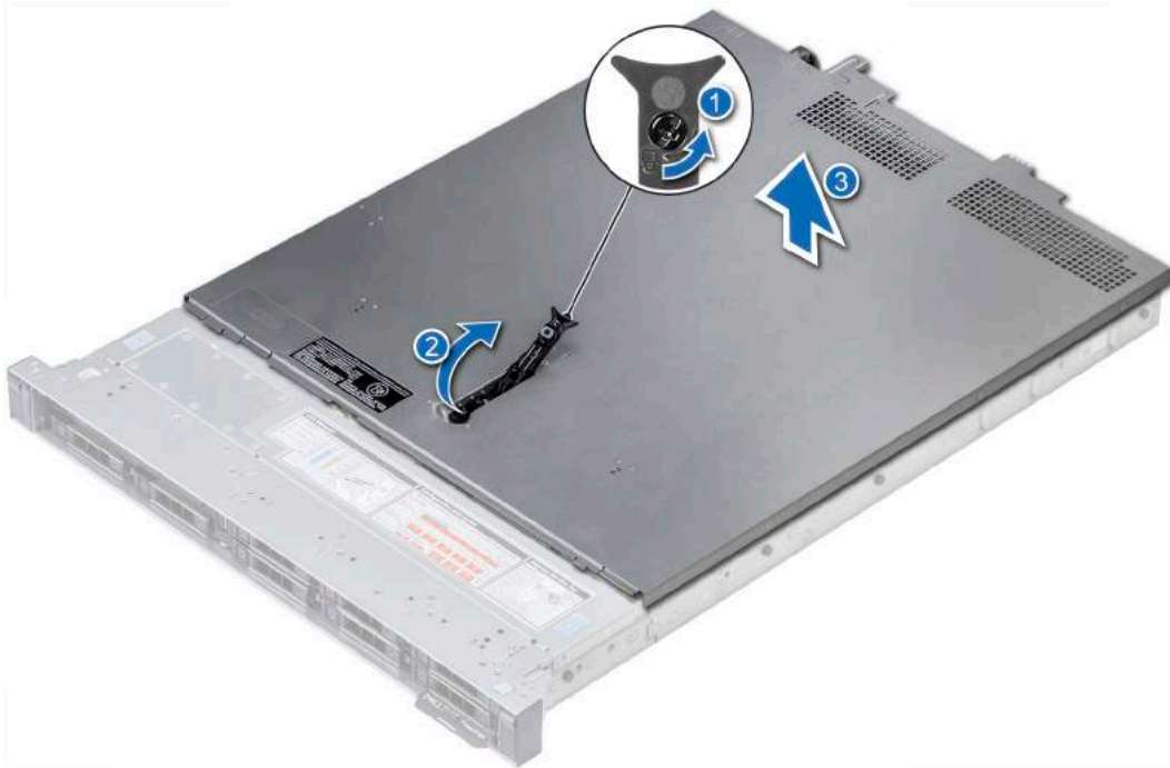
Figure 23. Removing the system cover
