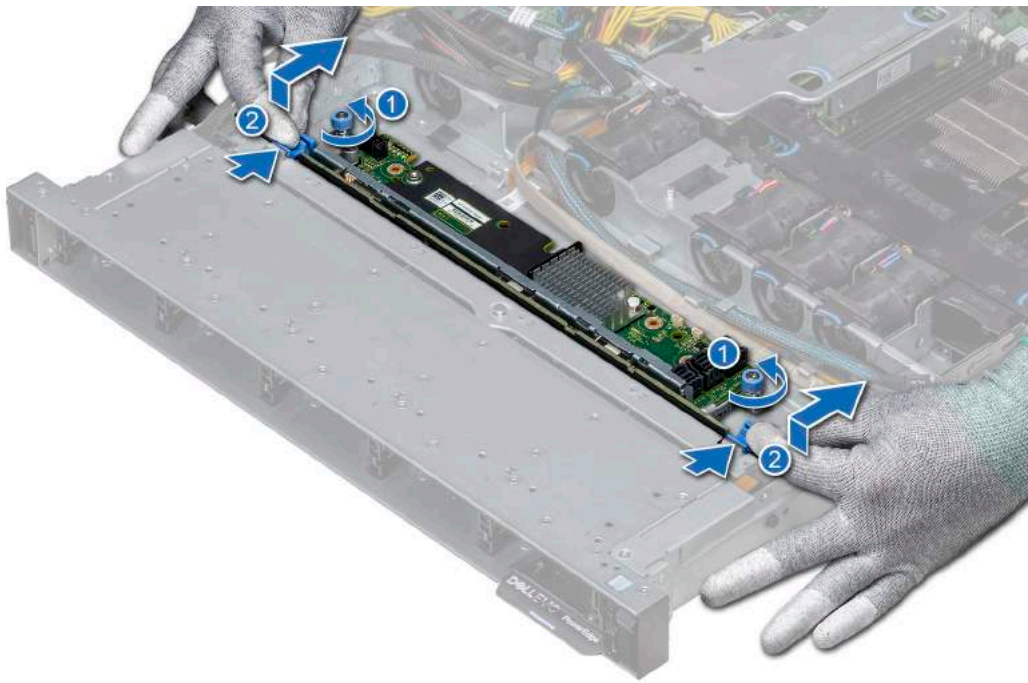
Figure 71. Removing the hard drive backplane
