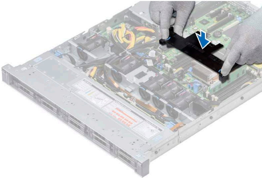
Figure 28. Installing the air shroud
