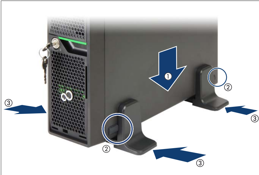
Figure 4: Placing the server on stabilizers
