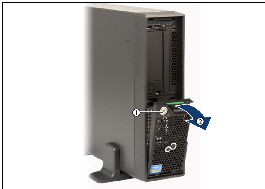
Figure 12: Removing the HDD cover
