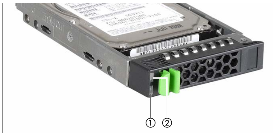
Figure 15: Indicators on the 2.5 inch HDD modules
