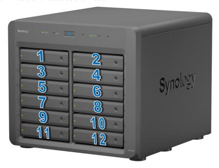
**Note:** If you want to create a RAID volume, we recommend all installed drives be the same size in order to optimize drive capacity usage.
