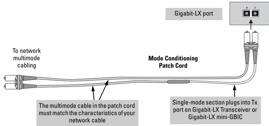
Make sure you purchase a patch cord that has LC connectors on the end that connects to the Gigabit-LX mini-GBIC, and has multimode fibers that match the characteristics of the multimode fiber in your network.
