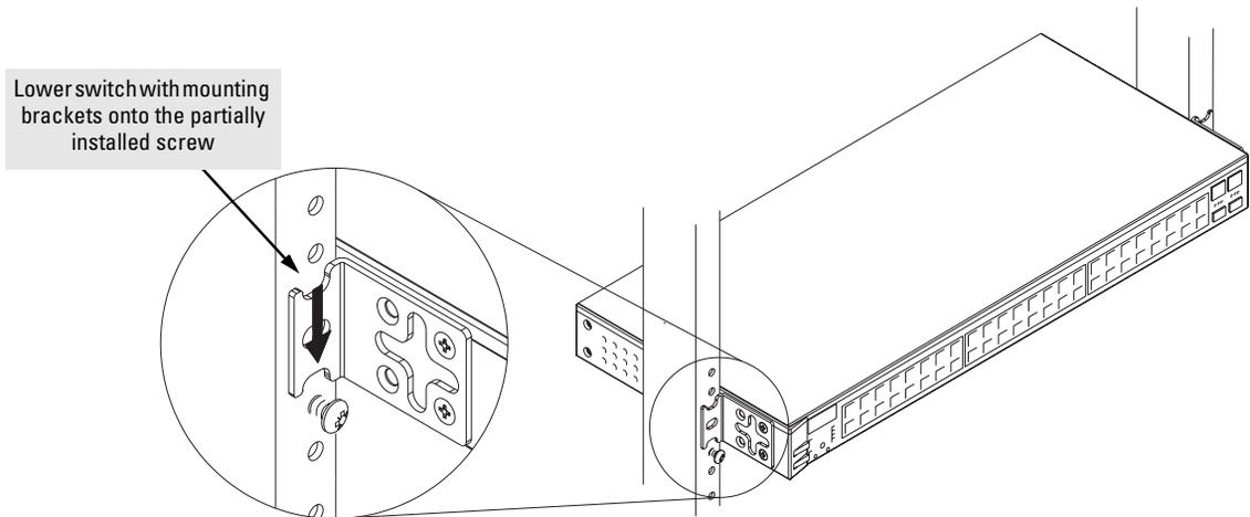
4. Install the other number 12-24 screw into the upper hole in each bracket. Tighten these screws.
