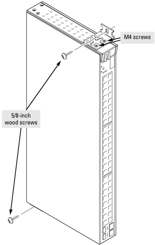
Note that the brackets are attached on opposite corners. This improves the stability of the switch on the wall.
