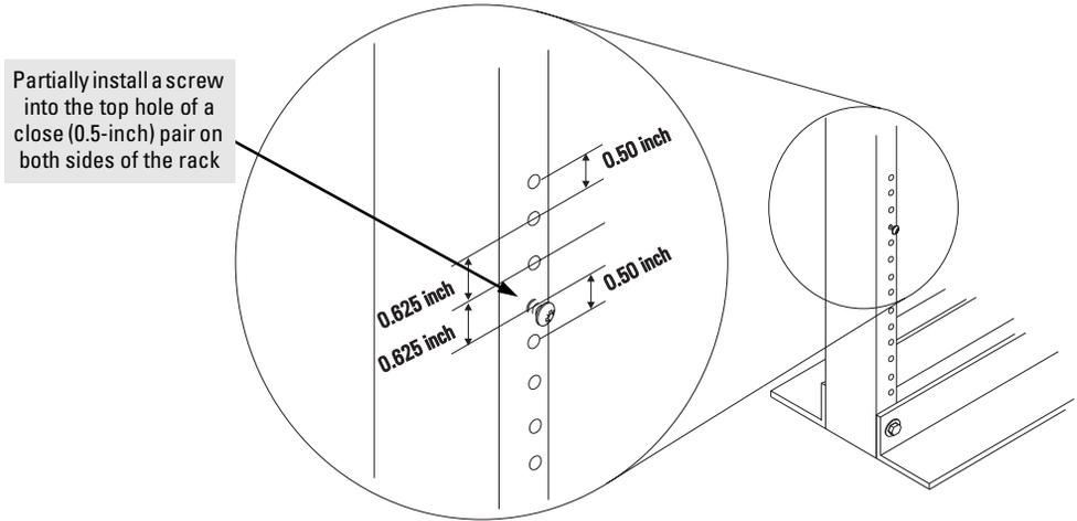
3. Place the switch in the rack and lower it so the notches in the bottom of the bracket slide onto the screws, then tighten these screws.
