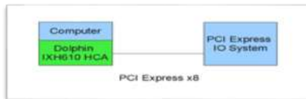
Illustration 2: IXH610 used to connect to a remote PCI Express IO System
