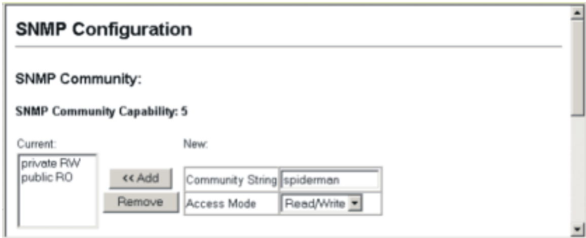
Figure 3-24 Configuring SNMP Community Strings
