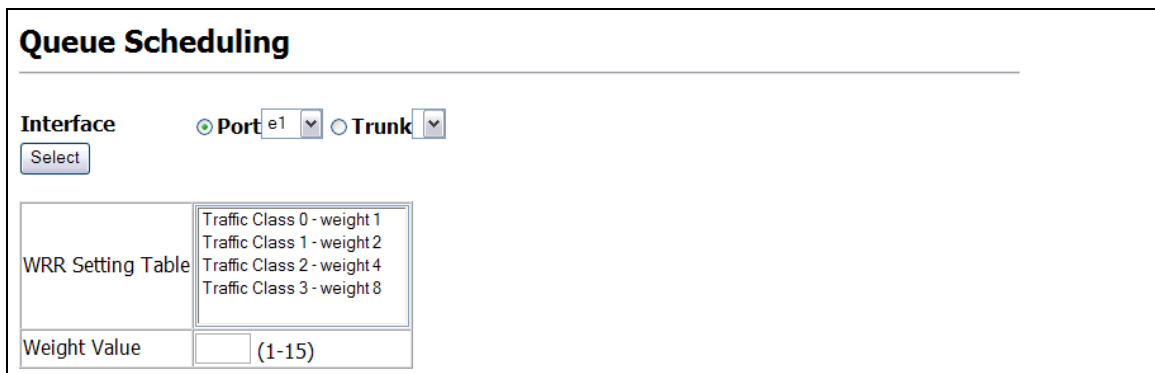
Figure 3-88 Configuring Queue Scheduling
