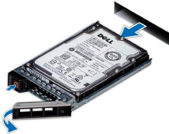
Figure 73. Removing a hard drive
