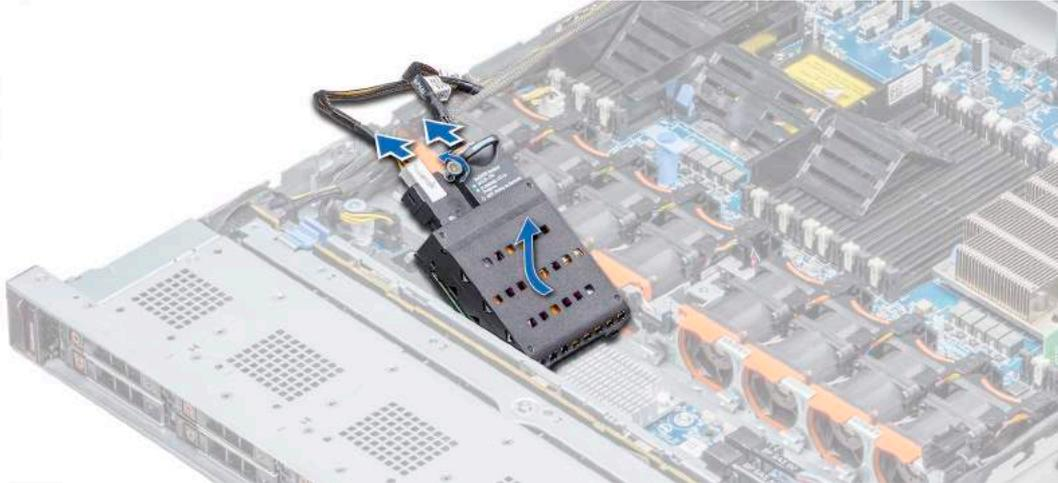
Figure 35. Removing the NVDIMM-N battery
