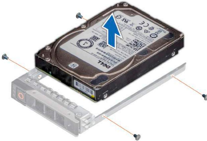
**Figure 75. Removing the hard drive from the hard drive carrier**
