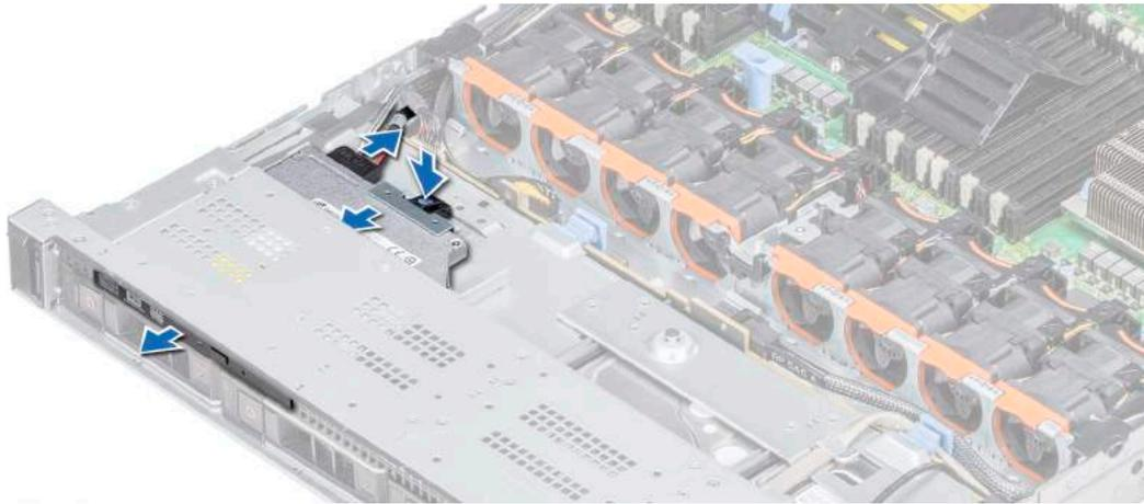
Figure 96. Removing optical drive
