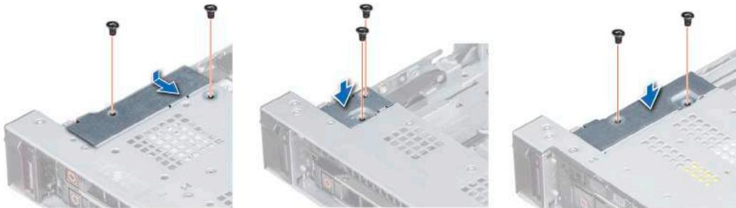
**Figure 108. Installing the cable cover**
