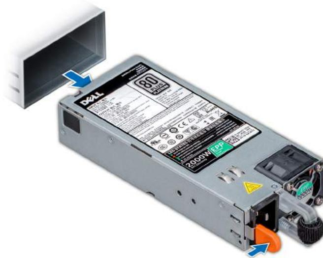
**Figure 100. Removing a power supply unit**
