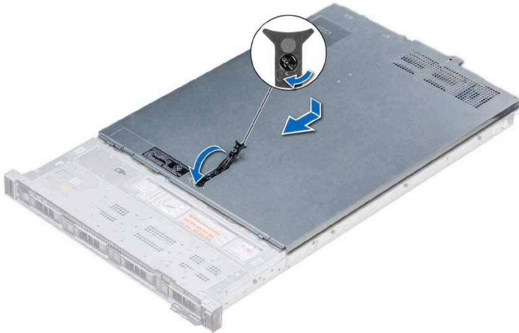
Figure 22. Installing the system cover
