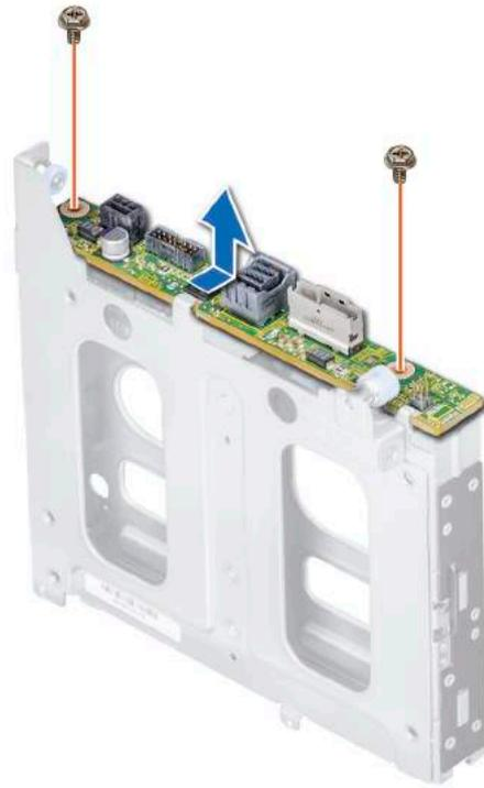
Figure 82. Removing the 2.5 inch hard drive back plane (rear)
