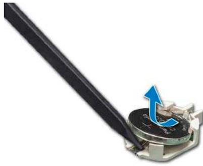
**Figure 92. Removing the system battery**
