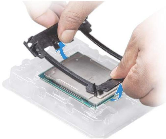
**Figure 39. Removing the processor bracket**
