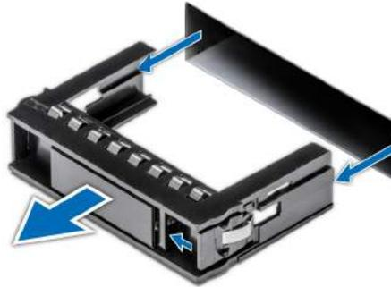
**Figure 71. Removing a hard drive blank**
