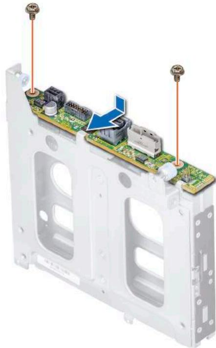
**Figure 84. Installing the 2.5 inch hard drive backplane (rear)**
