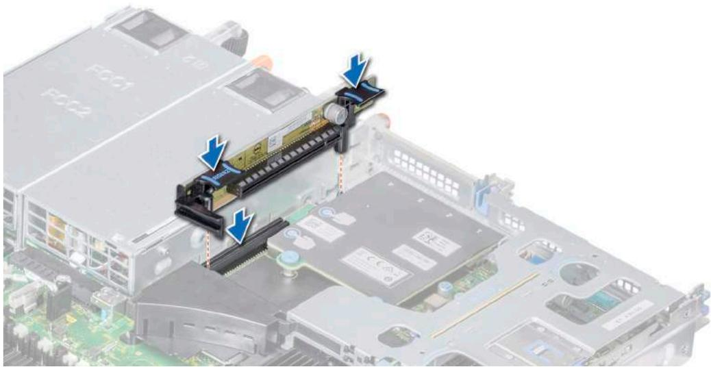
**Figure 50. Installing the expansion riser 2A**
