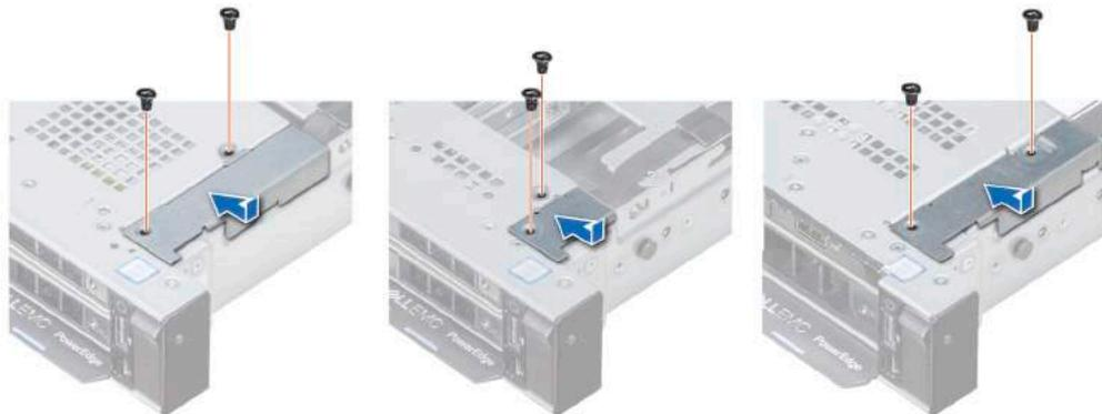
**Figure 112. Installing the cable cover**
