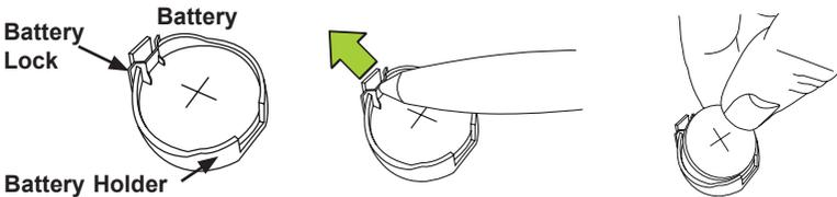
3. Using a tool such as a pen or a small screwdriver, push the battery lock outwards to unlock it. Once unlocked, the battery will pop out from the holder.
