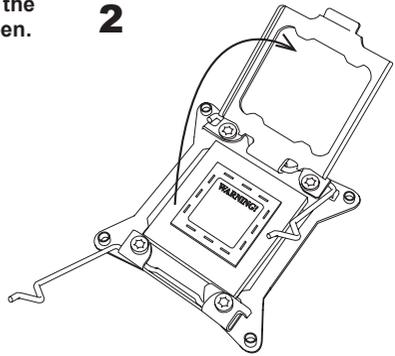
1. Use your thumb, and index fingers to loosen the lever and open the load plate.
