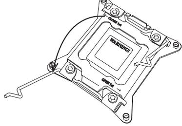
3. With the lever labeled 'Close 1st' fully retracted, gently push down on the lever labelled 'Open 1st' to open the load plate. Lift the load plate to open it completely.
