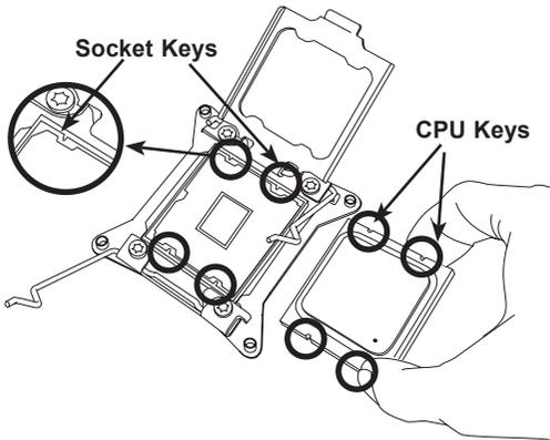
3. Once they are aligned, carefully lower the CPU straight down into the socket. (Do not drop the CPU on the socket. Do not move the CPU horizontally or vertically. Do not rub the CPU against the surface or against any pins of the socket to avoid damaging the CPU or the socket.)
