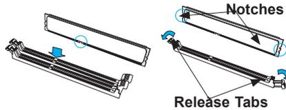
3. Align the key of the DIMM module with the receptive point on the memory slot.
