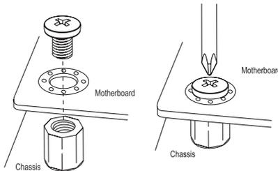
7. Repeat Step 5 to insert #6 screws into all mounting holes.
