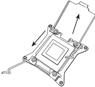
2. Using your thumb and index finger, hold the CPU on its edges. Align the CPU keys, which are semi-circle cutouts, against the socket keys.
