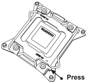
Press down on Load Lever labeled 'Open 1st'.
