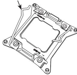
**3** Push down and lock the lever labelled 'Open 1st'.
