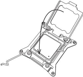
**2** Push down and lock the lever labelled 'Close 1st'.
