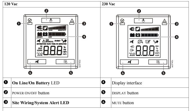
Note: Refer to "Feature Reference Guide" on page 11 in this manual for a detailed description of the front panel buttons and icons.
