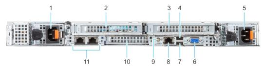
Figure 2. Rear view of the system
