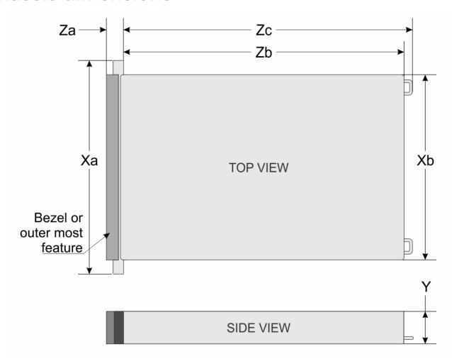
Figure 16. Chassis dimensions
