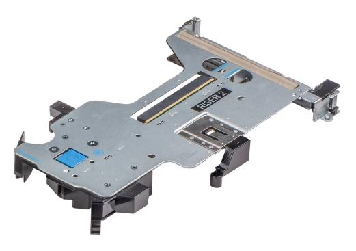
Figure 6. Slot 1 and 2 - Riser 2
