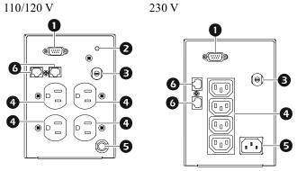
The top off white outlet helps to provide surge protection only. Equipment plugged into this 500 VA outlet should require surge protection, but should not require power during a utility power failure. The lower three outlets help to provide battery backup protection, as well as protection from surges.
