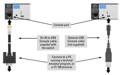
Figure 2-11. Connecting a console cable
