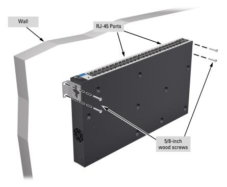
Figure 2-5. Wall mounting the 24-port and 48-port switches
