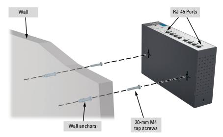
Figure 2-6. Wall mounting the 8-port switches
