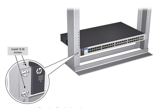
Figure 2-4. Mounting in a rack
