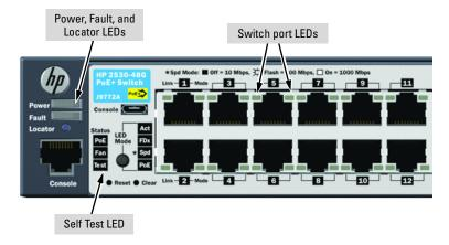
Figure 2-2. Checking the LEDs
