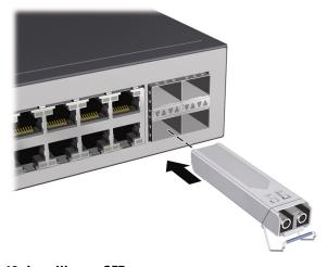
Figure 2-10. Installing an SFP
