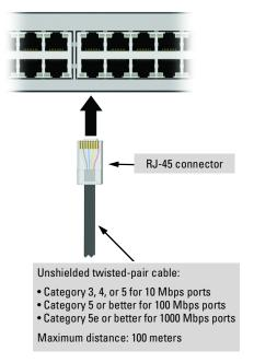
Figure 2-9. Connecting network cables
