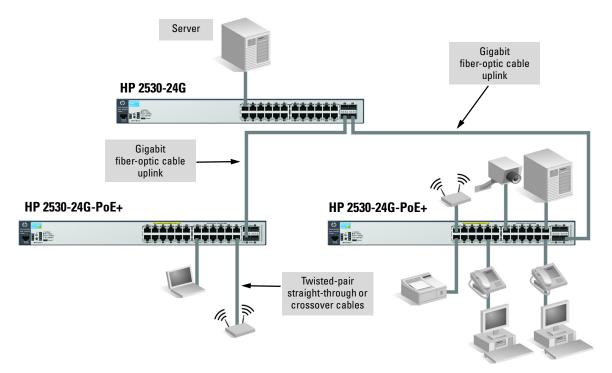
Figure 2-13. Segment network configuration with PoE switches
