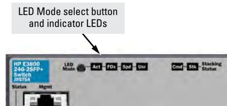
Figure 1-11. Example of Indicator LEDs on a PoE/PoE+ E3800 Switch
